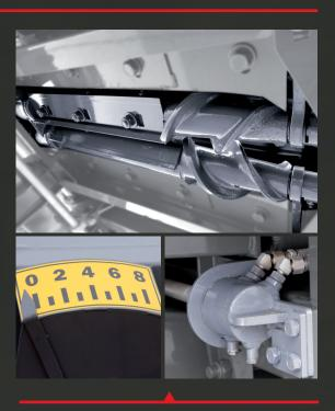
The deck plates are hydraulically controlled from the combine seat for easy adjustment. A clear indicator needle show the plates position to the operator.
